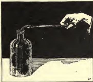
FIG. 57. The chlorin unites with the hydrogen of the turpentine, setting the carbon free.
