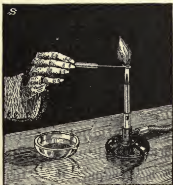
FIG. 51. The flame test.
