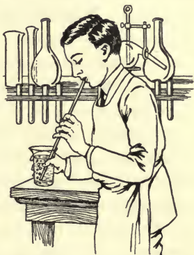
FIG. 84. The carbon dioxide unites with the limewater to form limestone.
