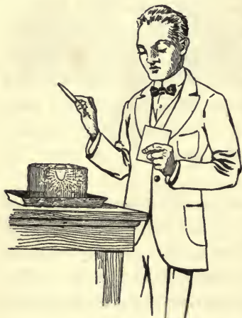
FIG. 59. Potassium in a cavity in a block of ice.
