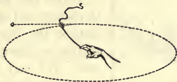
FIG. 136. A moving body tends to travel in a straight line.
