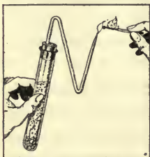
FIG. 36. Be careful not to light the gas until all the air has been expelled from the tube!
