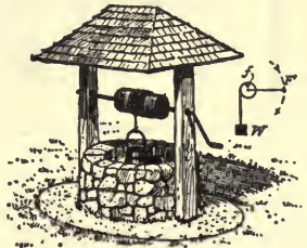
FIG. 210. A machine which gives an advantage in lifting power and in the direction in which the force is applied.
