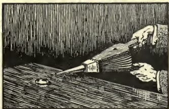
FIG. 160. An ice factory on a small scale. The evaporation of the ether takes up heat and freezes the watch glass to the board.
