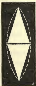
FIG. 175. Diagram to show how a lens convex on each side resembles two prisms with their bases placed together.
