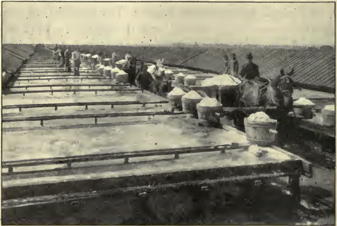
FIG. 48. Manufacturing salt in Syracuse, New York. The brine is pumped from deep wells and evaporated by the heat of the sun. The covers shown along the sides are turned down over the tables at night and during rains.
