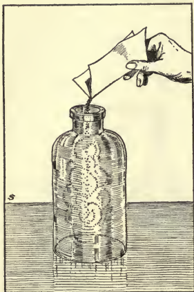
FIG. 56. When powdered iron is thrown into a jar of chlorin, a shower of sparks is produced.
