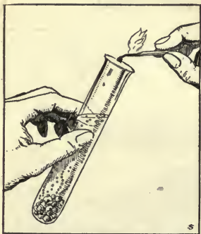
FIG. 35. Hold the test tube away from the body and with its mouth pointing away from the face.
