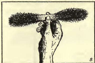
FIG. 188. The iron filings are attracted most strongly by the poles of the magnet.
