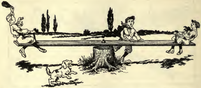
FIG. 213. A machine that gives an advantage in the speed with which the object is moved.
