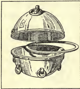
FIG. 120. The Magdeburg hemispheres used by Otto von Guericke in his famous experiment. The opening through which the air was exhausted is in the bottom of the lower hemisphere and is not shown in the illustration.
