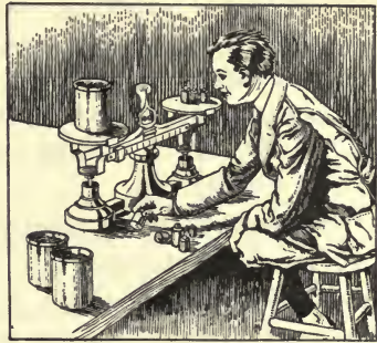
FIG. 99. Testing the water-holding capacity of soils.
