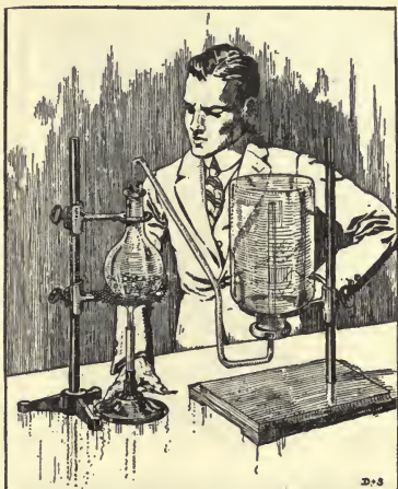
FIG. 113. Preparing and collecting ammonia.
